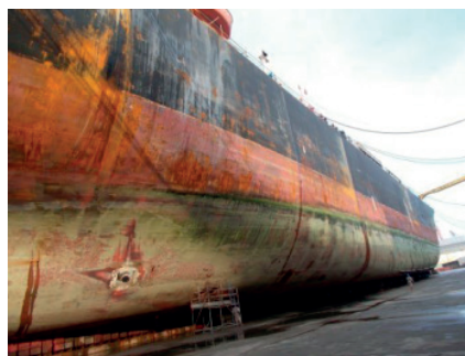
Performance on a 103,614 DWT LNG Carrier Vessel after 23 months in-service 77% activity > 3 knots, trading globally
